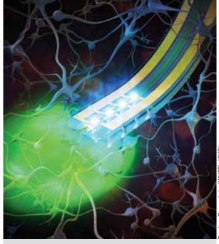
The wireless neural device developed by researchers at Washington University and University of Illinois features a dual-purpose probe that can stimulate through chemicals and light.
